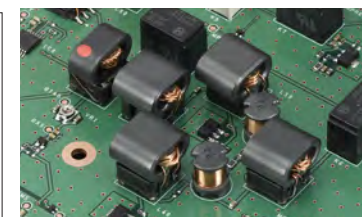
Transformer feedback RF Amp
