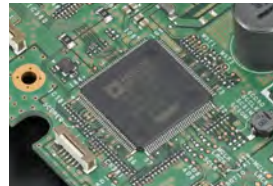
For band scope ADSP-21363 clock @333 MHz
