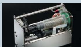
Inside the RF \mu -Tune unit
