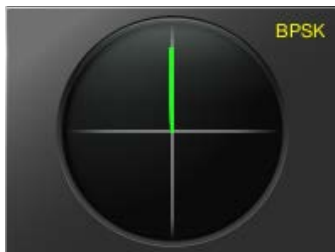
Non-modulated Carrier Signal
