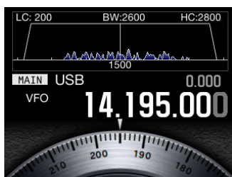
The selected band frequency Audio Band Scope & Dial Display
