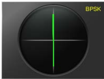
Tuned Correctly (BPSK Mode)
