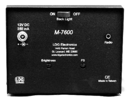
positive. External power is only required if use of the internal backlight is desired. The meter functions correctly otherwise without it.
