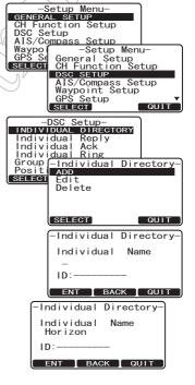
If a mistake was made entering in the name repeat pressing the Soft key until the wrong character is selected, then rotate the **CH** knob to correct the entry.
