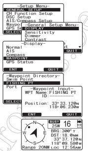
To stop the navigation to a saved waypoint, perform the steps 1 to 5 above, except selecting "NORMAL" in the step 5.
