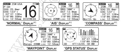
\*1: By default the COG in "NORMAL" and "COMPASS" displays and BRG in "AIS", "COMPASS", and "WAYPOINT" displays are set to "True", however this may be change to magnetic by following the steps in section "6.10 CHANGING COG TO TRUE OR MAGNETIC".
