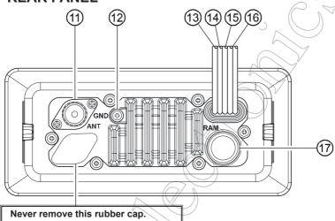
When this rubber cap is removed, the water resistance performance is lost.
